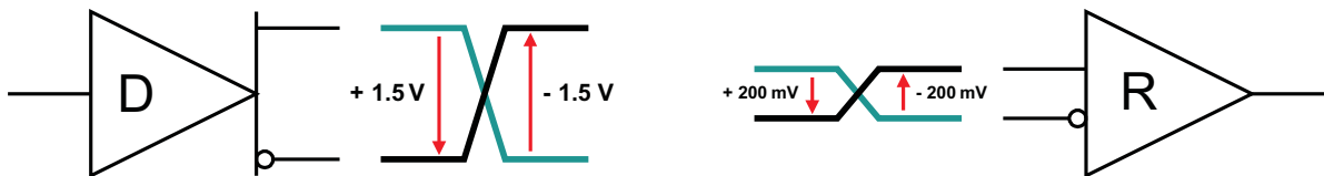
Figure 3. RS-485 Specified Minimum Bus Signal Levels
