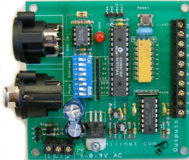
The DMX receiver module is designed to provide 8 consecutive channels of output from a standard DMX protocol input signal. The outputs may be configured to be digital (on-off), drive standard RC type servos, provide triggering outputs suitable for driving Triac lamp dimmer circuits- or a combination of any two of these. The base address of the module may be set in stages from 1 to 249 using the on-board setting switches (all address switches OFF for addresses 1 to 8 ).
