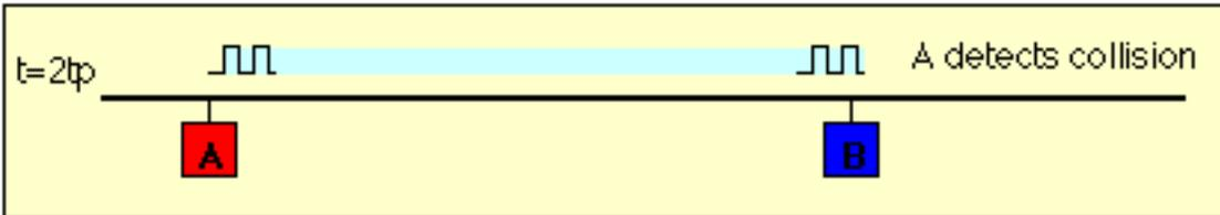
A short time later computer B also transmits. (In this case, the medium as observed by the computer at B happens to be idle too. After a period
