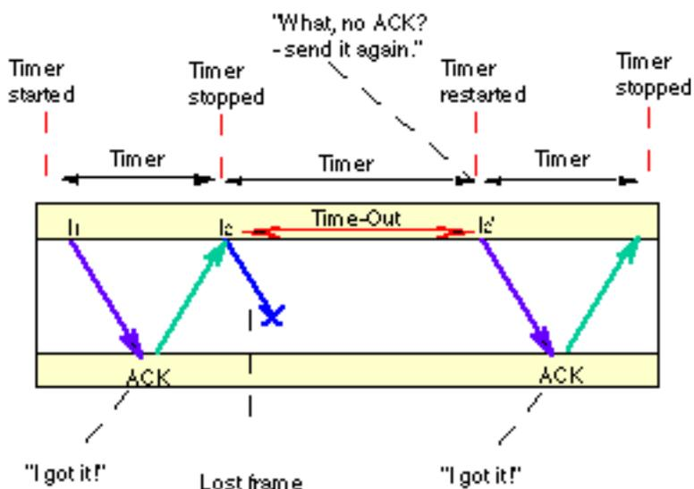
(e) Explain the operation of Automatic Repeat Request (ARQ) protocols and illustrate your drawing by showing how a Stop and Wait ARQ protocol may retransmit a single packet which was corrupted and discarded within a network. [5 marks]
