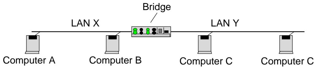
(a) The computer A sends a graphics file of size 10 MB simultaneously to computers B, C and D using Unicast packets constructed by the Universal Datagram Protocol (UDP). Calculate the utilisation of LAN X, given that each frame carries 1024 B of UDP payload data, and transmission is at 50 packets per second to each destination. [10marks]
