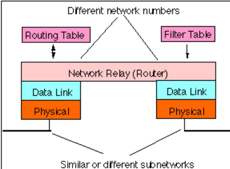
A router is an Intermediate System (IS) which operates at the network layer of the OSI reference model. Routers may be used to connect two or more IP networks, or an IP network to an internet.
