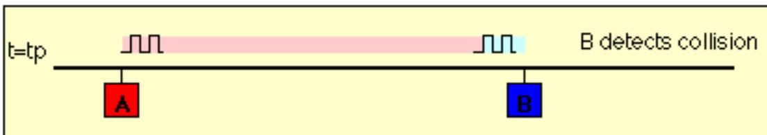
A second element of the Ethernet access protocol is used to detect when a collision occurs. Each transmitting node monitors its own transmission, and
