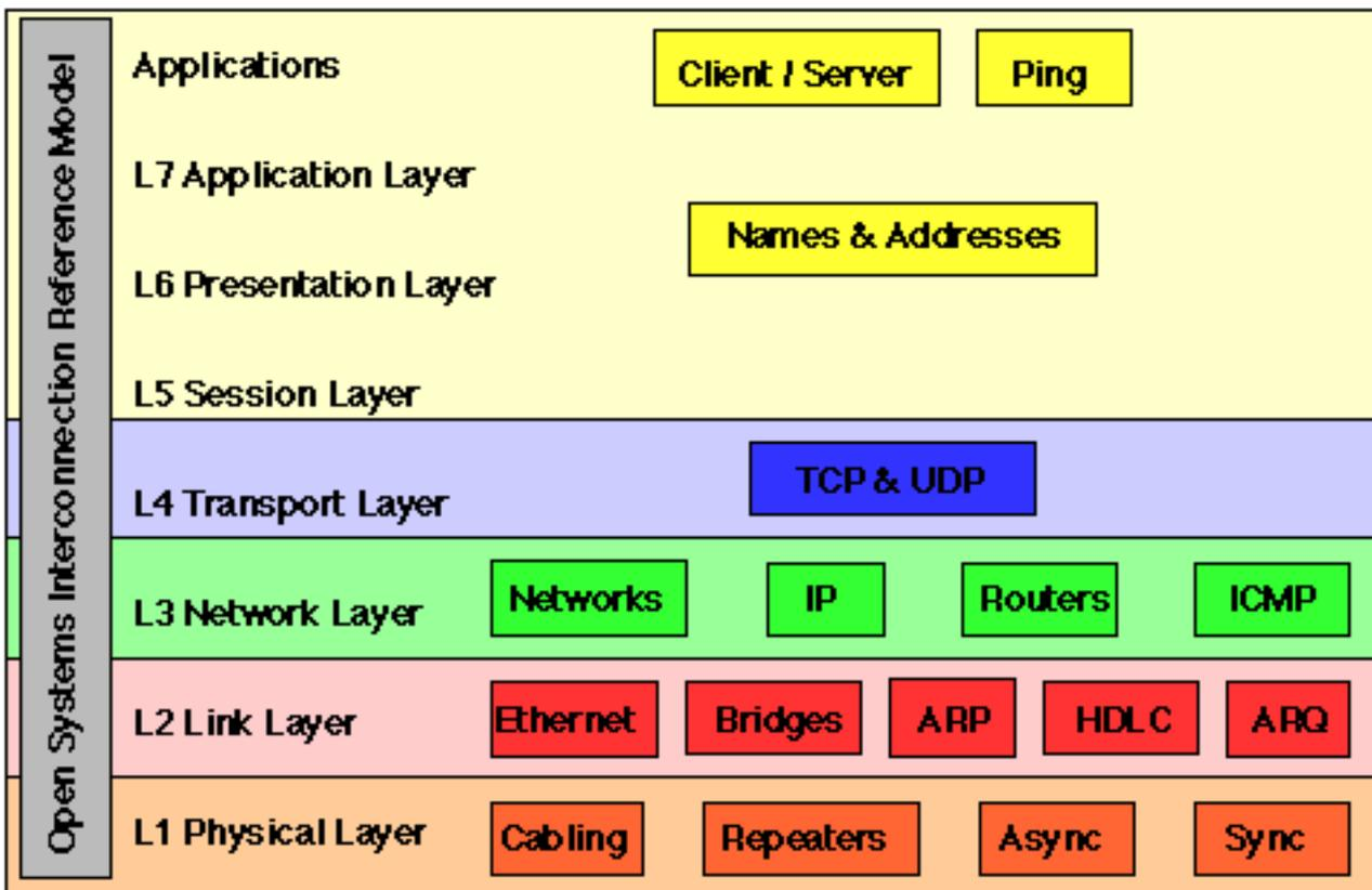
**Physical layer:** Provides electrical, functional, and procedural characteristics to activate, maintain, and deactivate physical links that transparently send the bit stream; only recognises individual bits, not characters or multicharacter frames.
