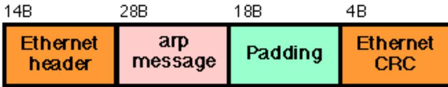
An arp message encapsulated in an Ethernet MAC frame (note the need for Ethernet Padding to ensure the minimum Ethernet PDU size)
