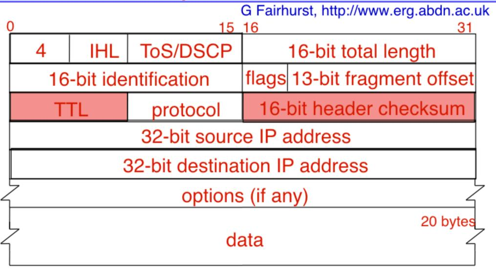
The TTL is decremented and discarded if zero The IP checksum is recalculated
