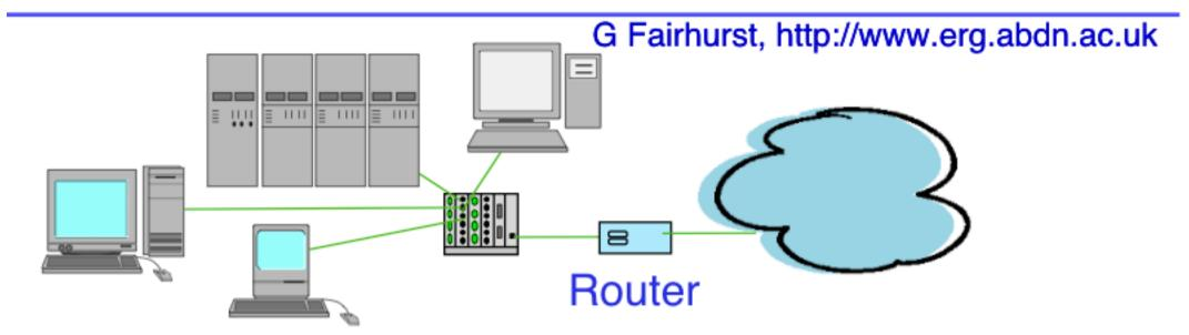
Addresses allocated to network as a *flat* address block e.g. Aberdeen University allocated 139.133.x.x/16 i.e. addresses start with the same address prefix e.g. 139.133.1.5, 139.133.208.1
